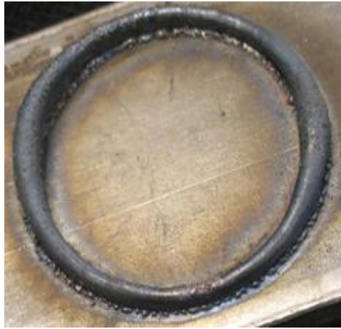
Figure 4.7. A part built using direct 3D layer
